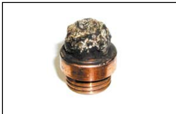
Low gas or no gas (Nozzle snuffing)
