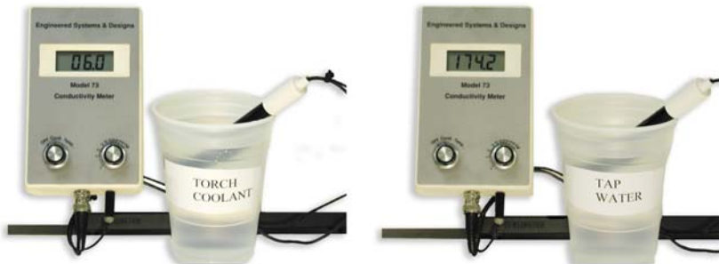
Figure 3 Measuring conductivity of coolant
